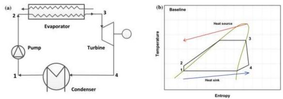
Figure 1. (a) ORC components and (b) Temperature (T) – Entropy (s) diagram
