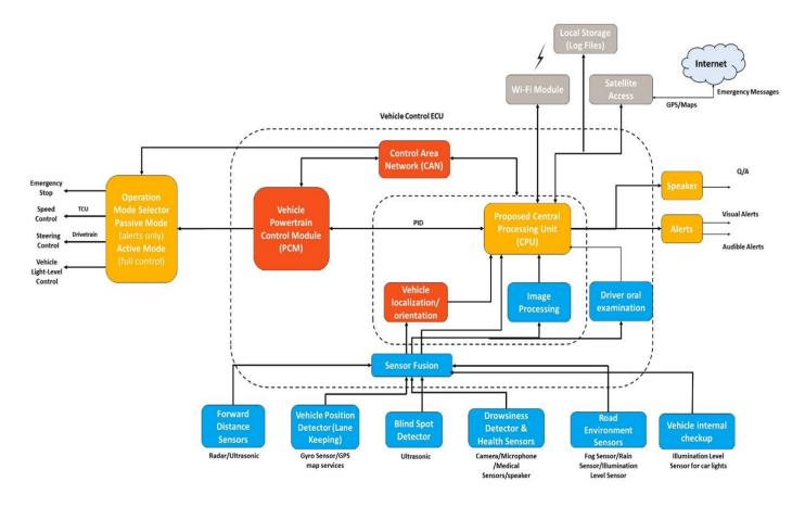
Figure 2 IDAS block diagram
