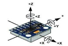
Figure 11 the rotation motion of Gyroscope in (x, y, z) axis
