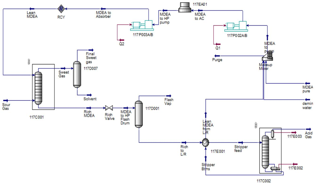
**Figure 4:** CO<sub>2</sub> Removal unit simulation using Aspen Hysys v11.
