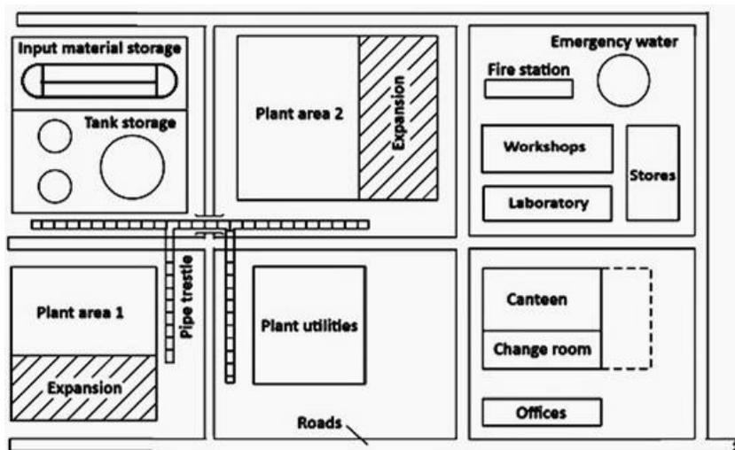
Figure 7: Plant layout for Acid Gas Removal.
