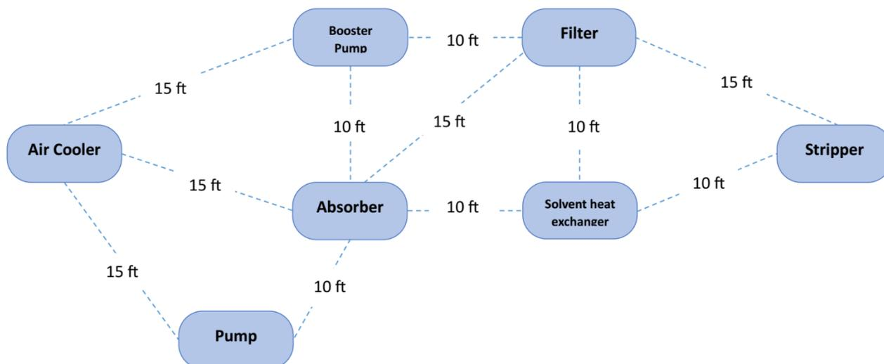
**Figure 6:** Equipment spacing of Acid Gas Removal plant.
