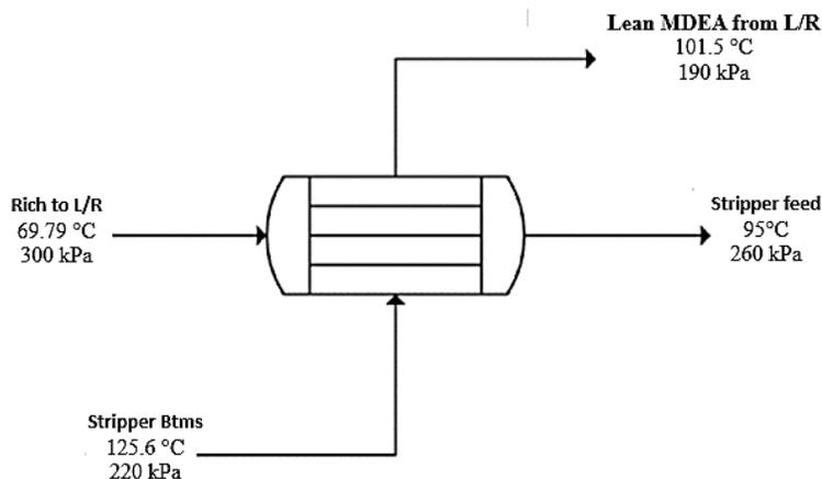
**Figure 5:** Illustrates the heat exchanger inlet and outlet streams.
