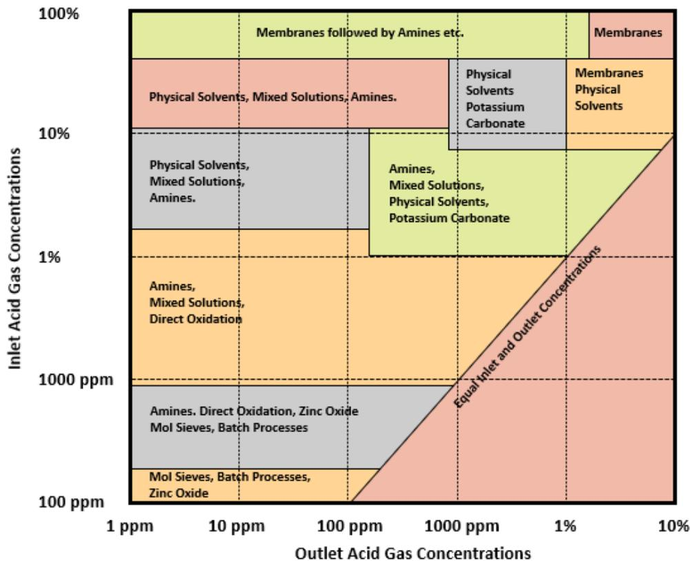
Figure 2: Matrix for Choosing Acid Gas Removal Technologies.
