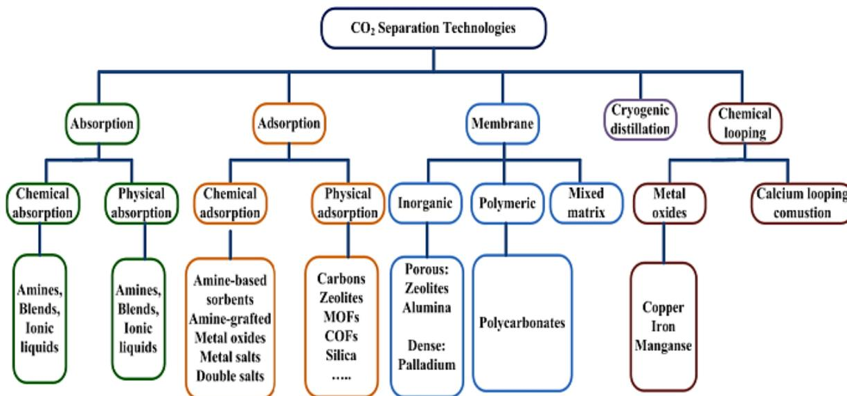
Figure 1: Different technologies used for CO<sub>2</sub> Separation Technologies from Natural Gas.
