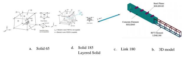
Fig. 2 Geometry and node locations for element types
