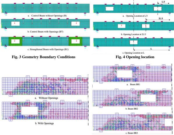
Fig. 5 Crack patterns for control beams
