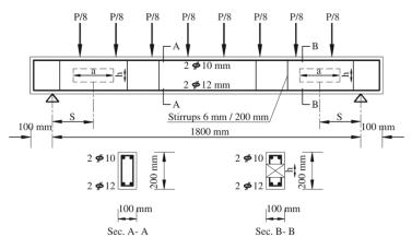
Fig. 1 Loads and steel reinforcement
