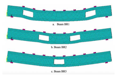
Fig. 7 Deformed shape for beams BR1, BR2, BR3
