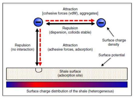
Fig. 4 The diagram shows the electrostatic interaction between charged NPs and shale (modified after [10]).
