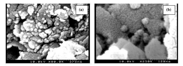
Fig. 1 SEM images of: (a) NPs plugging different pore throats, (b) aggregated particles plugging a pore throat (modified after [27]).
