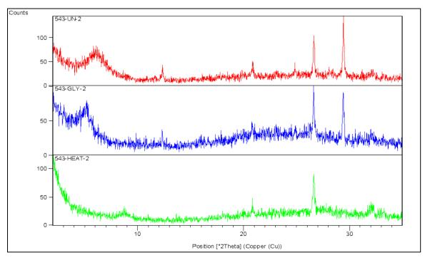
Fig.8 XRD analysis of the oriented, glycolated and heated phases of the Duwi formation shale sample.
