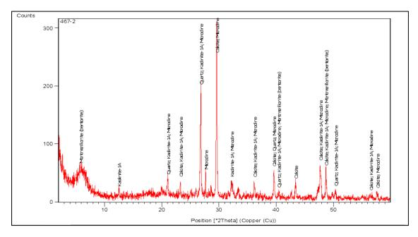
Fig. 6 XRD analysis of the Duwi Formation shale sample.
