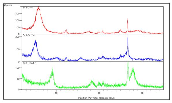
Fig. 9 XRD analysis of the oriented, glycolated, and heated phases of the Dakhla formation shale sample.
