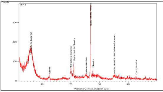
Fig. 7 XRD analysis of the Dakhla formation shale sample.
