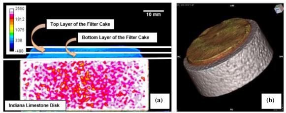
Fig. 3 CT scan images of the filter cake of the sample that have 0.5 wt% of Fe<sub>3</sub>O<sub>4</sub> NPs generated under static conditions at a differential pressure of 300 psi and 250°F: (a) 2D image with CTN-calibration scale, and (b) 3D cross-section. The calibration legend is in Hounsfield units (HU) (modified after [18]).
