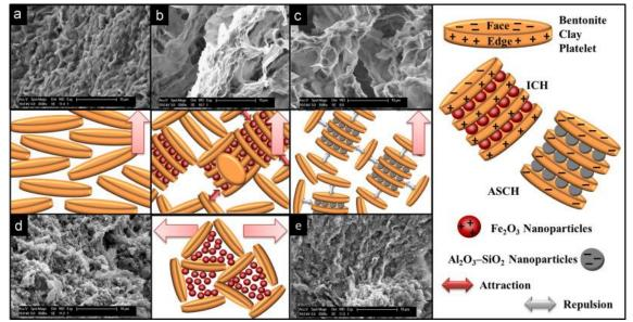
Fig. 2 SEM images of the filter cakes after LP/LT filter press experiments for different samples with the corresponding illustrations of bentonite clay platelet interaction (modified after [13]).
