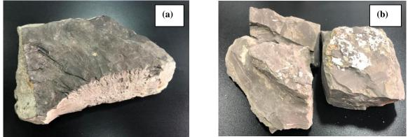
Fig. 5 Two shale samples; (a) Duwi Formation, and (b) Dakhla Formation shale.
